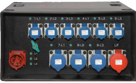
32-T1 32/3 Thru 6x 16/1 RCBO 3x 32/1 RCBO
