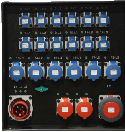
63-T2 63/3 Thru 2x 32/3 VTVS 6x 32/1 RCBO 12x 16/1 RCBO
