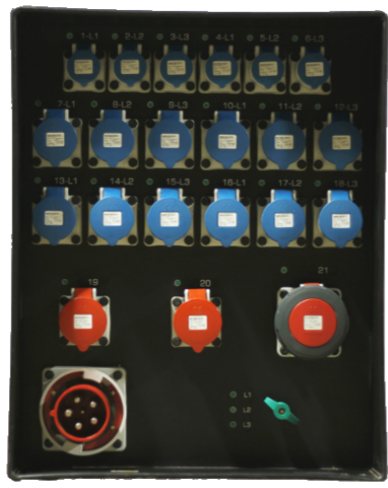
125-T4 125/3 Thru 1x 63/3 VTVS 2x 32/3 VTVS 12x 32/1 RCBO 6x 16/1 RCBO
